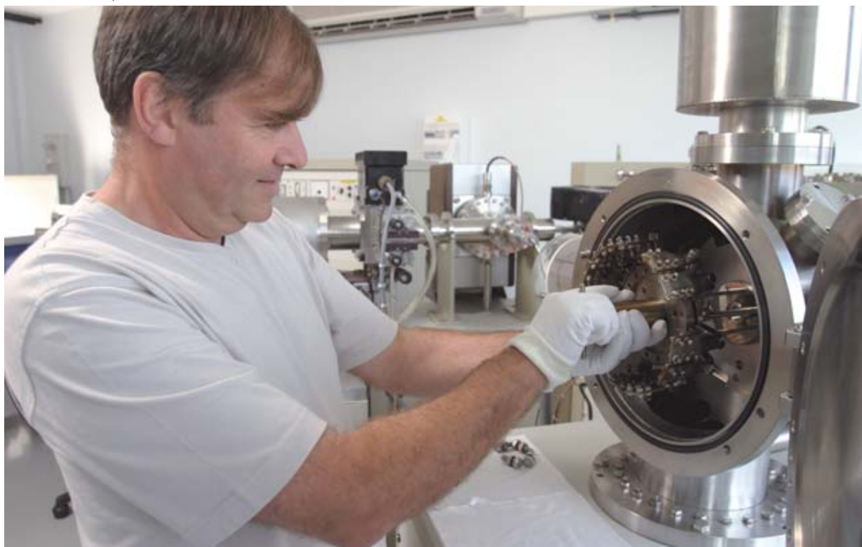
Thermal ionization mass spectrometer, allowing the very-high-precision analysis of uranium, and plutonium isotopes.
