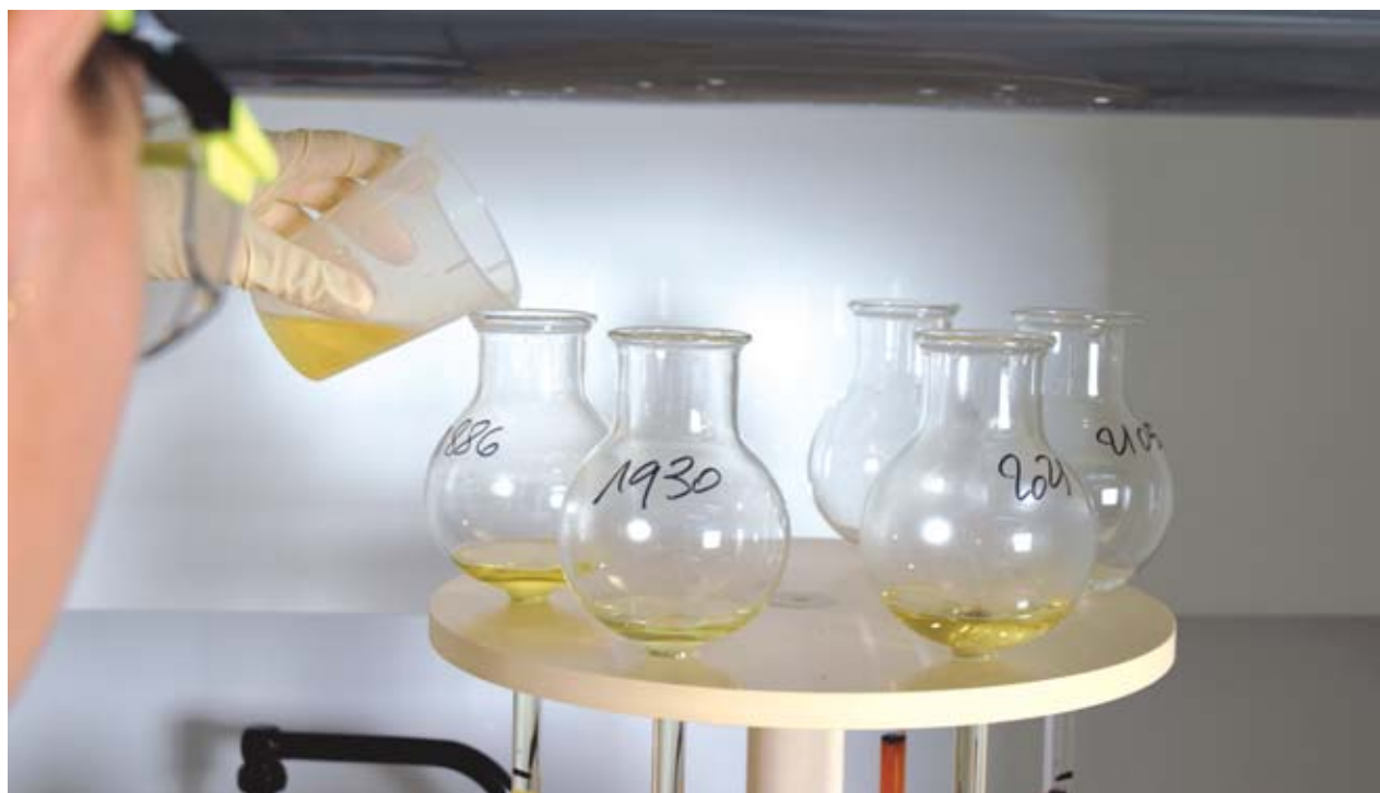
Preparing samples, for the purposes of radiological analysis. Environmental samples undergoing treatment: chromatography, for the purposes of extracting radionuclides .
